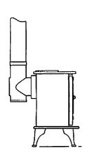
Rear outlet connected to top outlet by 'T' piece with cleaning door. This is the preferred method of installation.
