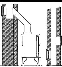
Top outlet with 45 degree bend sealed into masonry chimney with cleaning door on opposite side.
