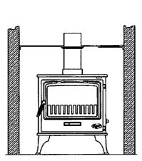
Top outlet through fully-sealed steel closure plate (fitted with cleaning door) into old, oversized, chimney with steel sealing collar.
