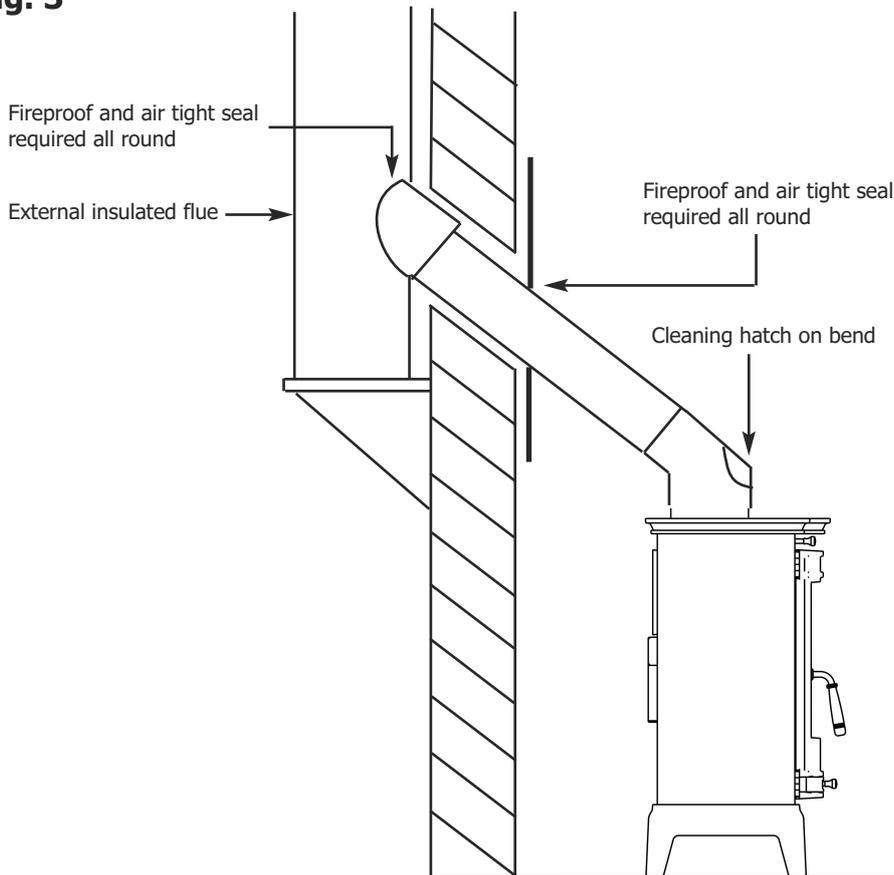
3.1.3 Rear flue outlet into chimney with sealing collar - figure 4
