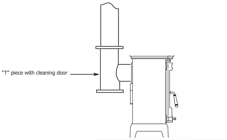
3.1.5 **IMPORTANT INFORMATION** - whichever method is used it is imperative that the route from the stove to the chimney terminal is completely air-tight, even very small air gaps can adversely affect the flue draught. Seal all joins with fireproof cement and / or heatproof rope. The entire construction should be made of durable fireproof materials.
