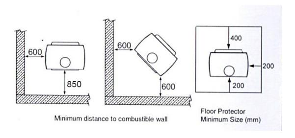
It is recommended that the stove be installed at least 600mm from combustible materials. However, any household furnishings should be at least 1000mm away as they could be adversely affected by heat.
