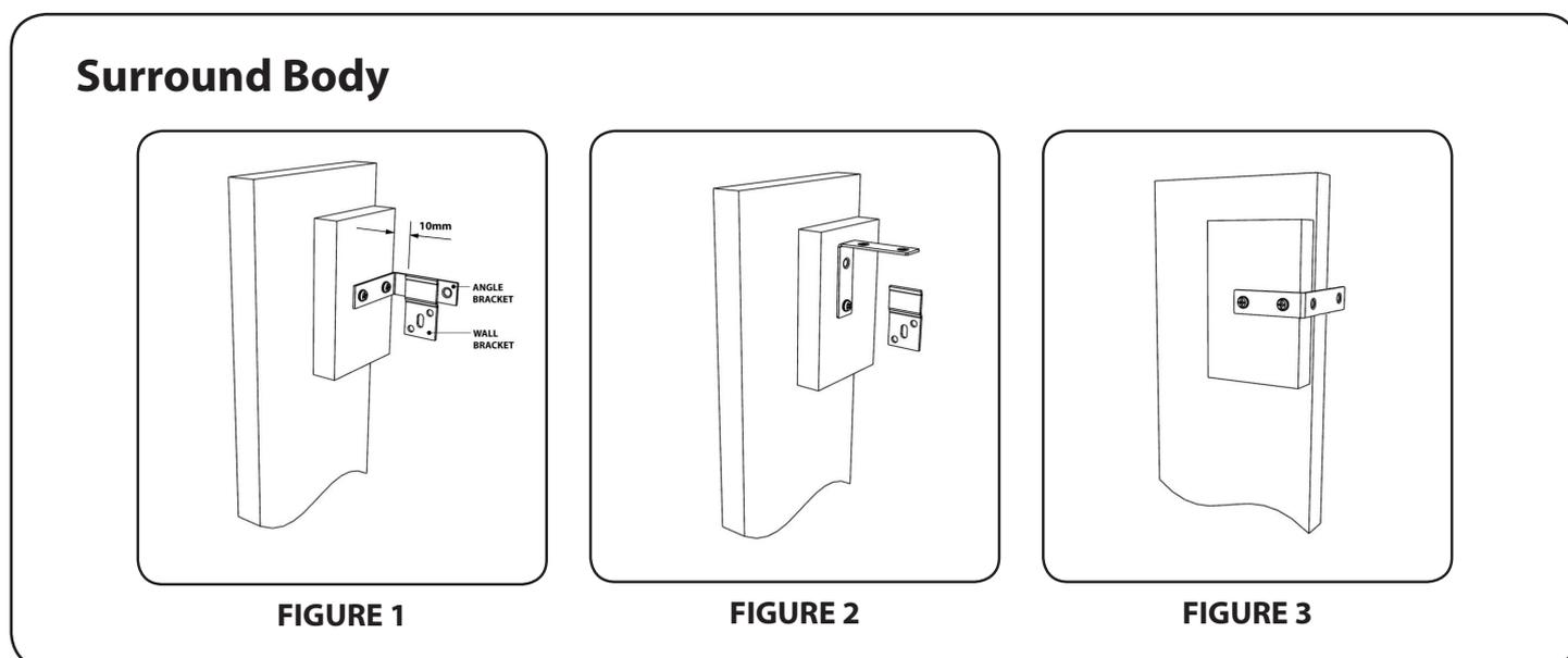
The tops of the leg sections have angle brackets fitted for securing direct to a wall surface. These fixing brackets will prevent the surround from detaching itself from the wall.
