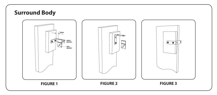
The tops of the leg sections have angle brackets fitted for securing direct to a wall surface. These fixing brackets will prevent the surround from detaching itself from the wall.
