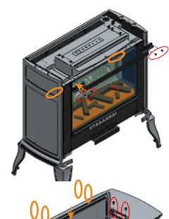
10) Screw the 1x M6 screw back into the top of the front casting.
