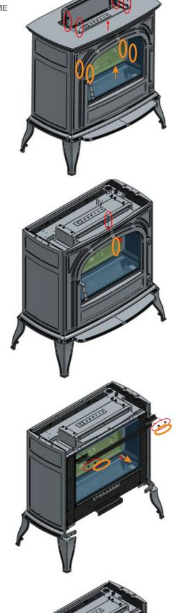
Carefully lift the glass up and out of the appliance and place safely on a soft, flat surface.
