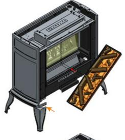
Ensure the glass is supported at all times! We strongly recommend protective gloves are used when handling glass.
