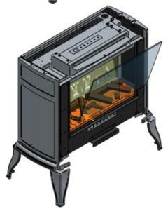
9) Screw the 4x firebox screws back into place, securing the glass and the retaining to the appliance.
