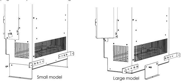
Secure the appliance in the desired position by screwing down through the brackets on the sides or rear of the appliance as shown below
