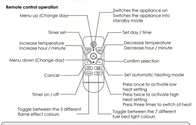
**NOTE:** The heater should be powered on using the Main Power switch before it can be operated using remote control
