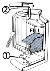
Place two or three firelighters close together, or screwed-up the back of the grate and light them. When they are burning well gently fill the fire with dry fuel, close the door and set the air control slides to the 'high' (right) position. When the fire is burning well, move the controls to the lowest practical setting.
