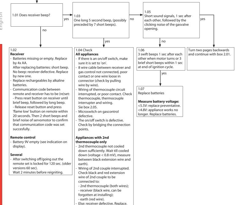
Malfunction search diagram atmospheric gas-fired heating appliance with electronic ignition: Starting up cycle.
