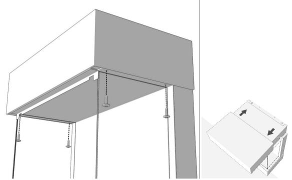
• Remove the four screws and slide the top forward.
