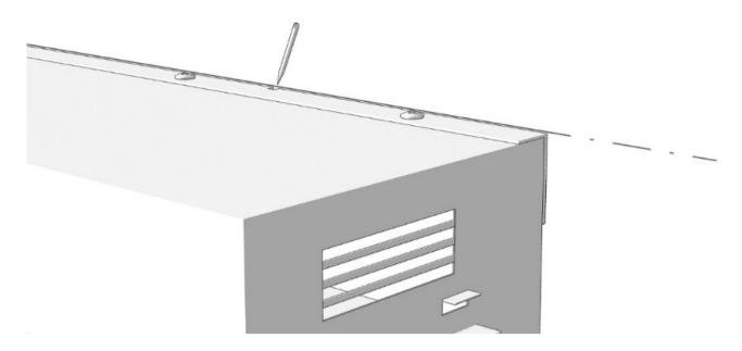
Remove the 13mm screws and top bracket from the fire. Using it as a template mark the fixing holes on the wall, drill the holes with an M10 bit and fit the rawl plugs. Using the 60mm screws fix the bracket to the wall.
