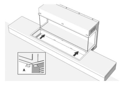
b. Using four of the 13mm screws secure the base to the fire along the side flange and fit the décor trim
