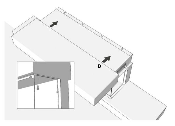
e. The chimney breast requires a baton to be fitted to the wall above the fire using three M10 x 50mm rawl plugs and 60mm screws. Use an M10 bit to drill the holes. The baton must be fitted from the top of the fire to the bottom of the baton, dead centre so the chimney breast can comfortably slide over the fire and line up to the pilot holes either side of the baton.
