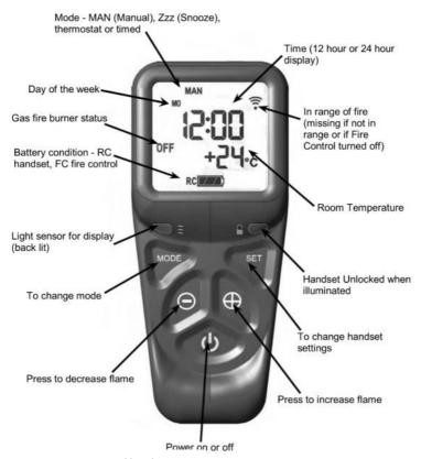
Fig.4 Remote control handset
