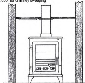
Typical Rear Flue Installation with clean out door
