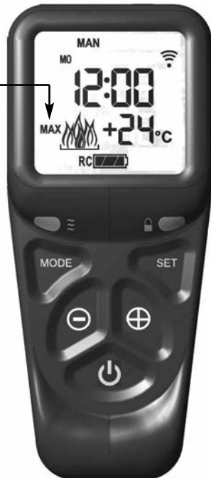
Fig. 45 - "MAX" & large flame symbol displayed
