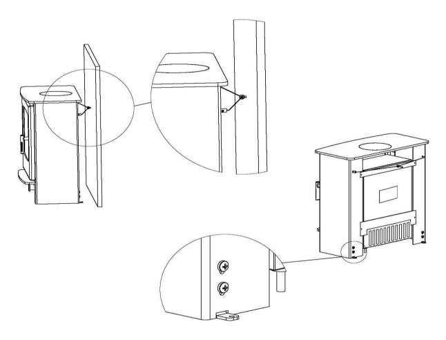
The floor fixing points also provide adjustment to level up the product when placed on an un-even surface. Front Adjustment is provided by two concealed bolts (under the base).
